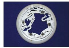
With all the features of the 5B Universal Base the 5BI Isolator Base allows any or all 800 Series MX Detectors to be upgraded to incorporate bi-directional short circuit isolation. Implemented on every detector, the 5BI can ensure that no detector is lost on a system in the event of an open or short circuit
