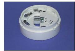
The 801RB provides dual relay contacts for signalling external devices on MX addressable systems. A very low operating current even when the relay is energised enables the relay base to be used without any additional power. The dual contacts are under the control of a programmable output, through the powerful cause and effect software.
